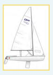
**420s** are fast, fun sloop rigged double-handed (two sailors!) boats that are very popular in youth programs around the country. The 420s used by intermediate and intermediate / advanced sailors have a main and jib. The C420s are rigged with spinnakers and trapezes for use by performance and racing instruction, for ages 13-17 and a minimum weight of 105 lbs.
